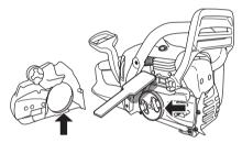
Regularly check that the brake band is at least 0.024 inch (0.6 mm) thick at its thinnest point.
